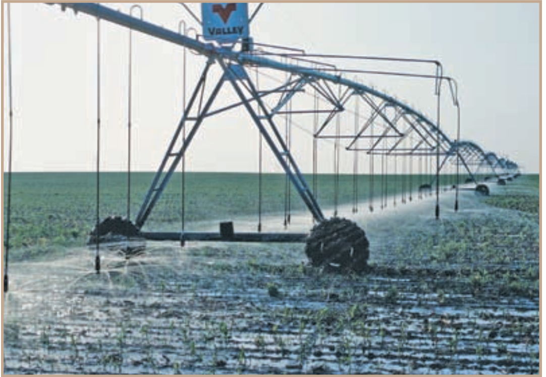
An example of a center-pivot irrigation system. (Courtesy of the Natural Resources Conservation Service; photo by Tim McCabe)
