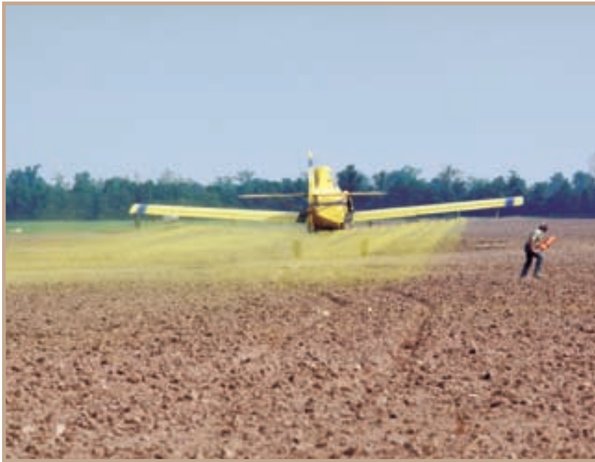
An example of an airborne application of pesticides in a field. The airplane flies very low to the ground to avoid wasting the chemical in the wind. (Courtesy of the U.S. Department of Agriculture; photo by Tim McCabe)
