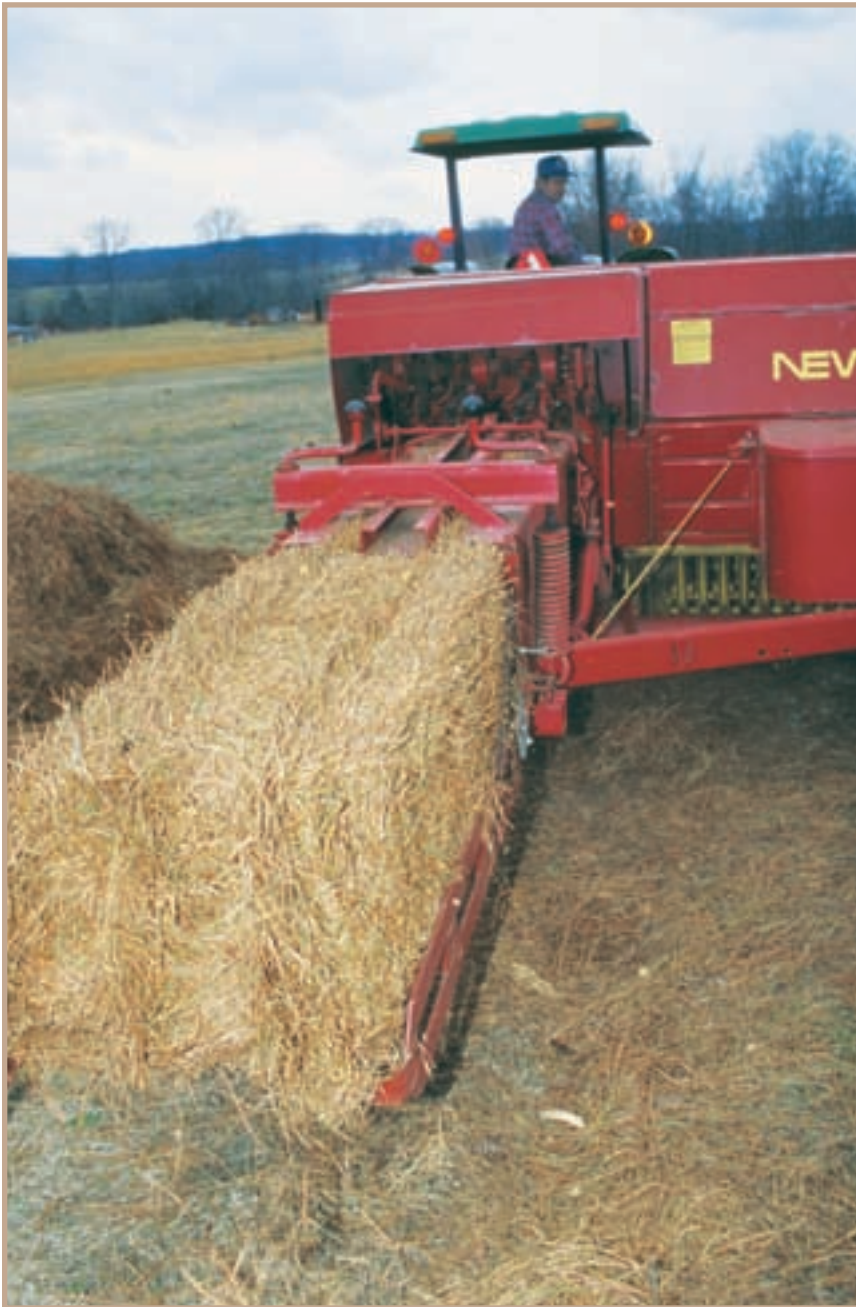
Rectangular bales of hay produced from a baler. (Courtesy of the U.S. Department of Agriculture; photo by Ken Hammond)
